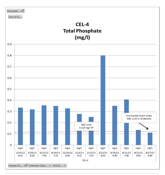
Field Trials of PhosFilter Adsorption System For Reduction Of Total Phosphorus (TP) In Residential Stormwater Pond. Numerous Modifications/Adjustments Were Made To The Intake Screen (Algae/Debris Ingestion Issues) Over Several Months. System Fully Operational In Late July 2013. August 27, 2013 Sample Was In Compliance With NNC For First Time In 18 Months. Samples Collected From Pond Outfall To Canal Receiving Water.
